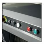
Front control panel Motorized adjustment of the upper belt height (height of loaves). Next to the front panel controls, a timer accurately records your working time.
