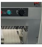
Variable speed drive Allows the cutting speed to be adjusted to suit the type of bread.
