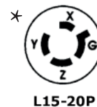
* Plug Configuration • NEMA L15-20P
