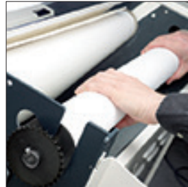
Forming belt Ultra-quick belt change without disassembling the machine.
