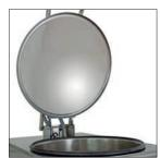
Watertight lid Fitted with a removable hermetic seal, the Tradilevain ensures a high degree of stability in the sourdoughstarter.
